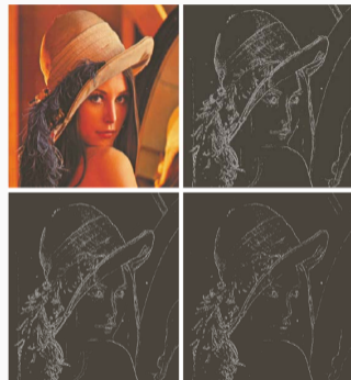
Figure 56: RGB edge detection. (1, 1): Original. (1, 2): Gradient in RGB color vector space ( F ). (2, 1): Gradients computed on per RGB component, and then added. (2, 2): Difference between (1, 2) and (2, 1).
