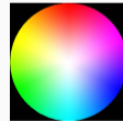
Figure 17: Chromaticity modeled as a unit polar coordinate chart ( \rho, \theta ) where fully saturated colors are at the boundary ( \rho = 1 ), and the angle \theta represent the wavelength, and thereby the hue.
