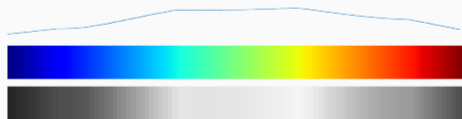
Figure 25: A gradient of jet , and the lightness component of the CAM02-UCS colorspace.
