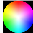
Figure 17: Chromaticity modeled as a unit polar coordinate chart ( \rho, \theta ) where fully saturated colors are at the boundary ( \rho = 1 ), and the angle \theta represent the wavelength, and thereby the hue.
